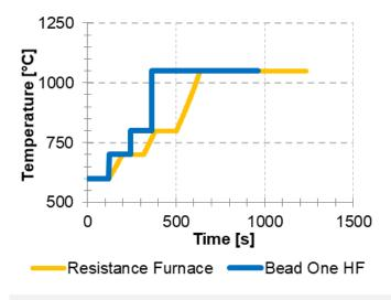
**Figure 2:** Heating profile of the Bead One HF in comparison to a resistance furnace. It is also possible for the Bead One HF to set ramps with different slopes in order to slow down the heating.
